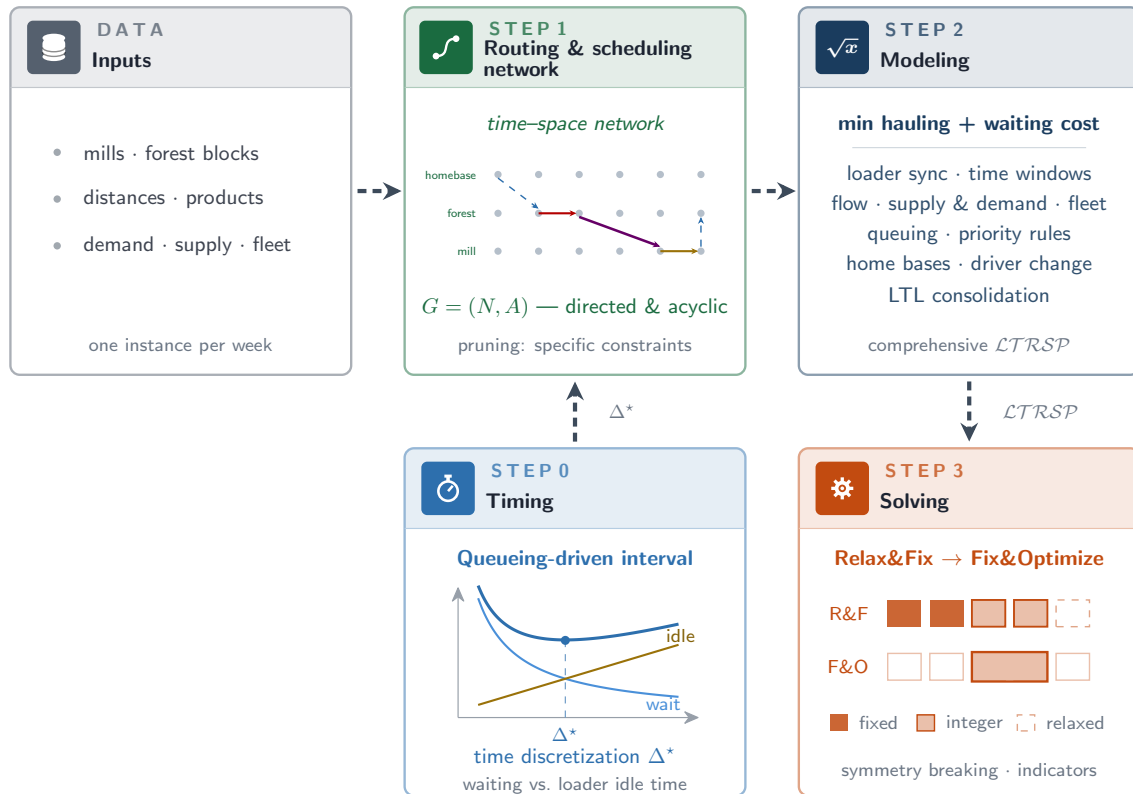
Figure 3: Overview of the kernel component: a queueing-driven time interval determines the granularity of a time-space network, on which the optimization model is formulated and solved using a Relax & Fix – Fix & Optimize decomposition (Abdellaoui et al. 2026b).
