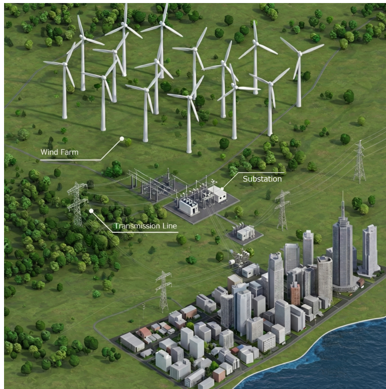
Figure 1: Configuration of an onshore wind power system.
