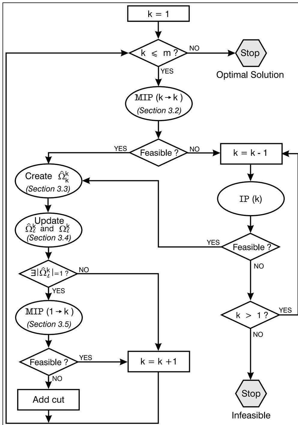
Figure 1: A diagram of the solution approach
