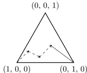
**Figure 1: Belief state dynamics for a 3-state machine  $i$  in the simplex  $\Delta(\{1, 2, 3\})$ .** Dashed arrows show a sample realizations of the belief state evolution under  $A_t^i = 0$  for three time steps and the solid arrow shows a sample realization of the belief state evolution under  $A_t^i = 1$
