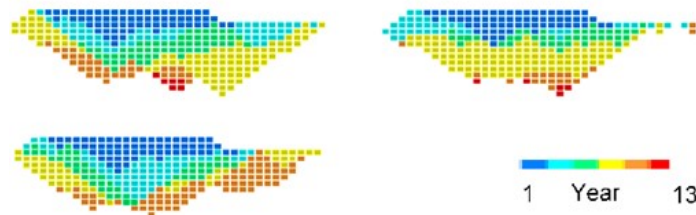
Figure 7: N-S cross section of production schedule Mine 1; a) base case (top left), b) branch 1 (top right), and c) branch 2 (bottom left).
