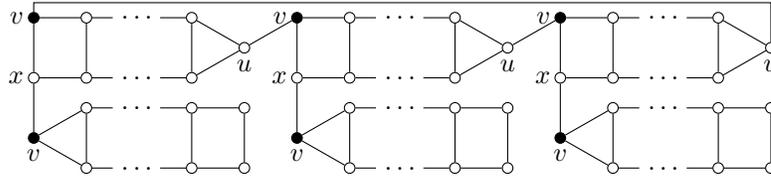
Figure 2: Graph  $G_{k,r}$ , when  $k$  is odd and  $r = 3$ .
