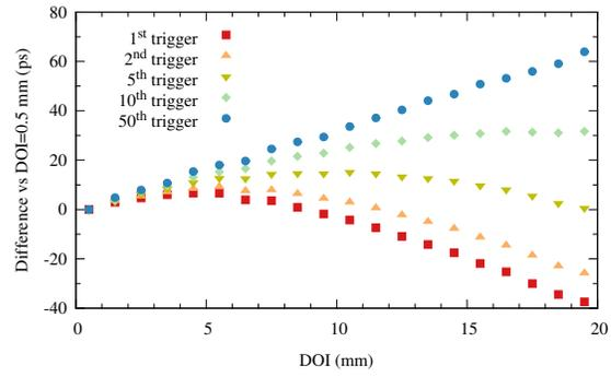
Figure 2: Bias for five  $k^{\text{th}}$  arrival time triggers when a Typical SD is in coincidence with another Typical SD where interactions occur at a fixed DOI of 0.5 mm.
