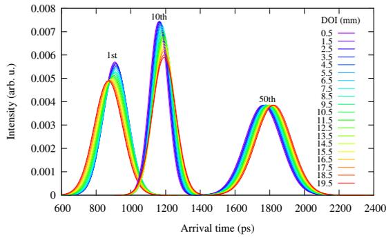
Figure 1: Distributions of three primary triggers arrival times (1<sup>st</sup>, 10<sup>th</sup>, 50<sup>th</sup>) in a single Typical SD as a function of DOI.
