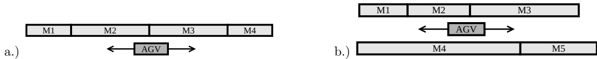
Figure 1: AGV handling materials in a single-row layout (a) and a double-row layout (b).
